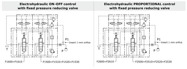
Proportional control kit, mechanically retrooperated, allows the maximum precision of positioning, limiting the hysteresis. The control is operated with PWM control of the current. PWM frequency suggest: 60-80 Hz
