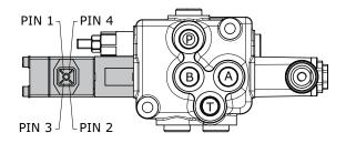
**CONTROL in A e B** = connect PIN 1 - 4 and 2 - 3
