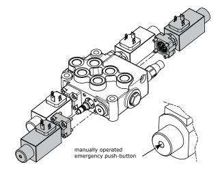
The H036 and H037 direct electric controls come as two kits each including a: spring, solenoid and adapter.
